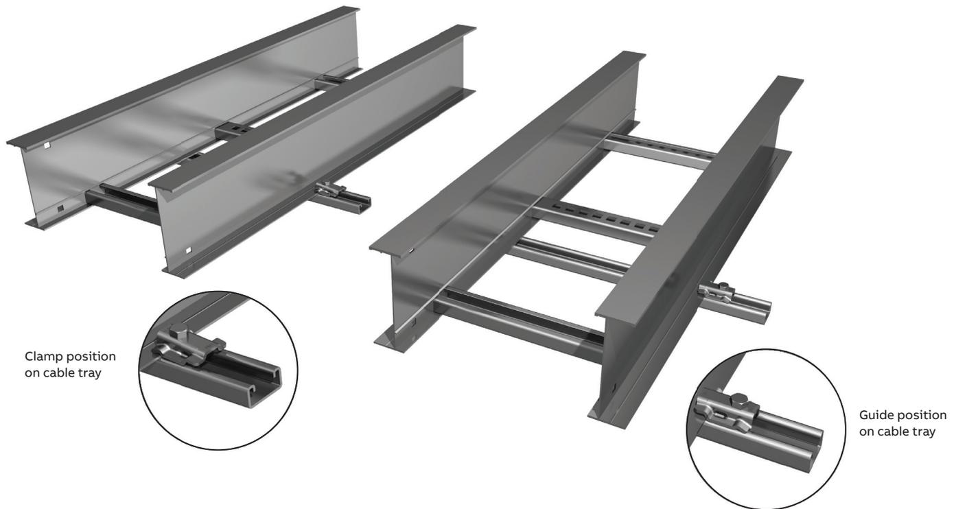
Stock one design for all hold-down and expansion needs. The innovative new combination hold-down/expansion-guide clamp from Thomas & Betts can be used on all series of T&B Cable Tray, regardless of side rail thickness.
